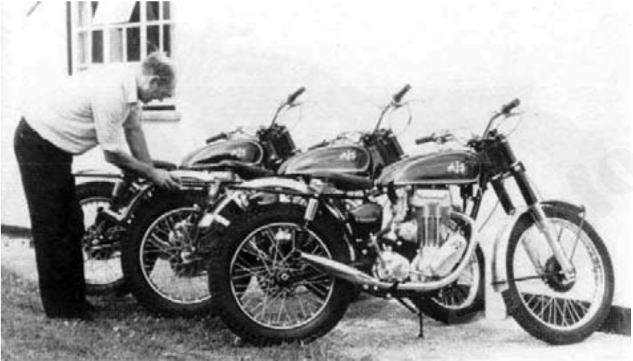
A trio of 1959 model 16C trials machines with their small brakes and shortened subframe. Virtually their final form.
